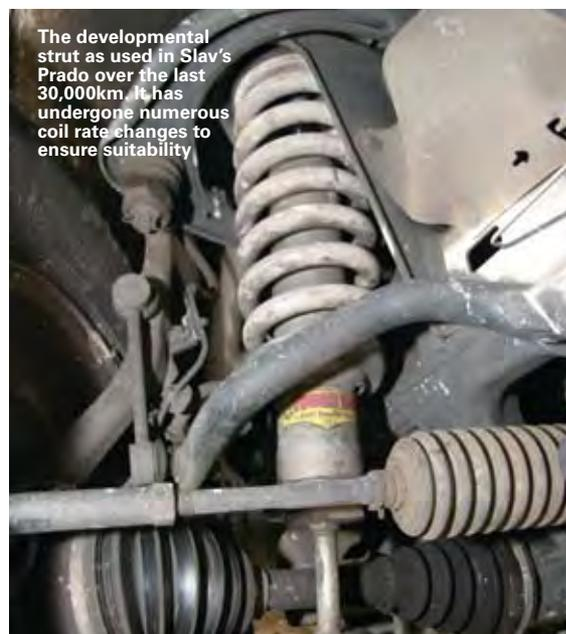
The developmental strut as used in Slav's Prado over the last 30,000km. It has undergone numerous coil rate changes to ensure suitability
