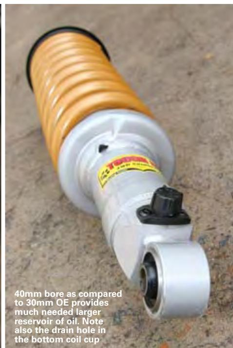
40mm bore as compared to 30mm OE provides much needed larger reservoir of oil. Note also the drain hole in the bottom coil cup
